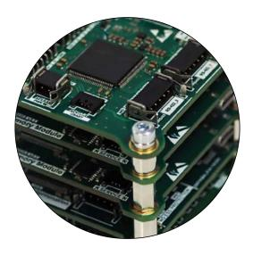
The OBC-K1 is a flight-proven, reliable solution for suborbital rockets. With a dedicated enclosure, it is capable of withstanding even the harshest environmental conditions. 7 different modules have been developed so far. Custom module design possible.
