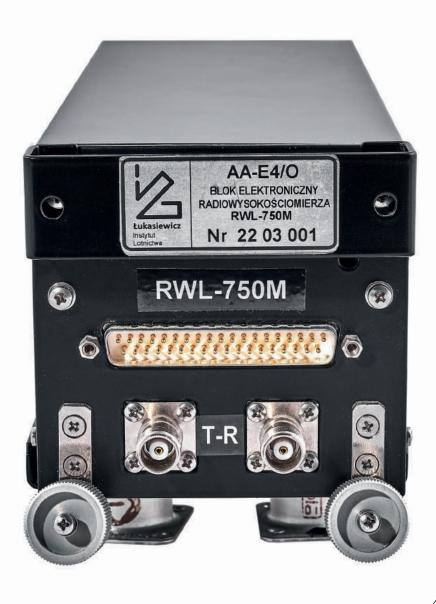
A Radio Altimeter (RADALT) is an electronic instrument used to measure the distance between an aircraft and the terrain directly below it
