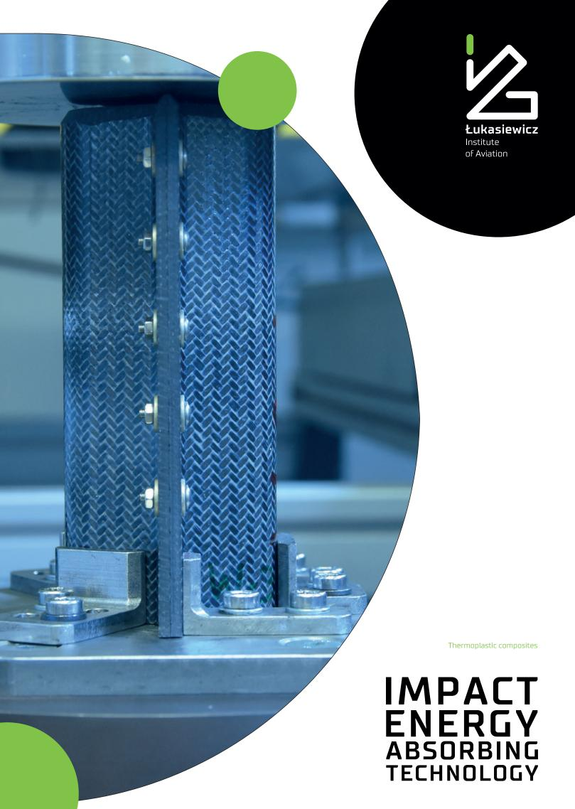
Łukasiewicz – Institute of Aviation has developed an innovative technology for the use of thermoformed composite materials, resulting in the ability to produce impact energy-absorbing components. Composite energy absorbers may find applications in various industries, primarily aviation and automotive.
