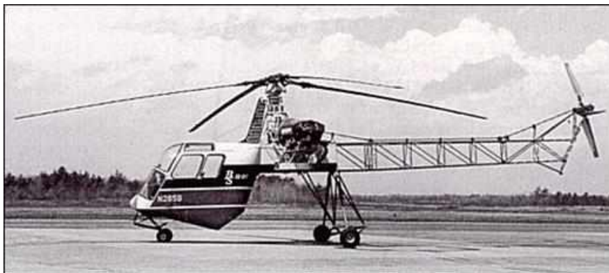
Fot. 2. Omega BS-12D Utility Flying Crane
