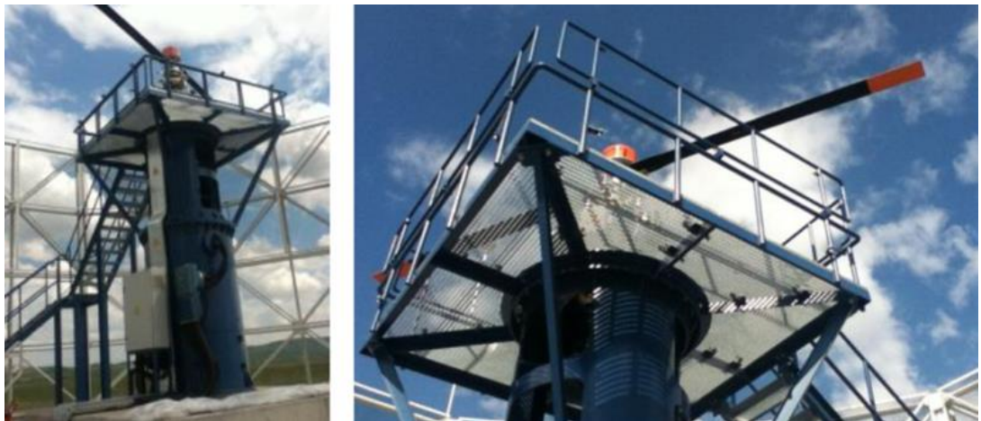
Fig. 1. The TAI whirl tower system [2]
