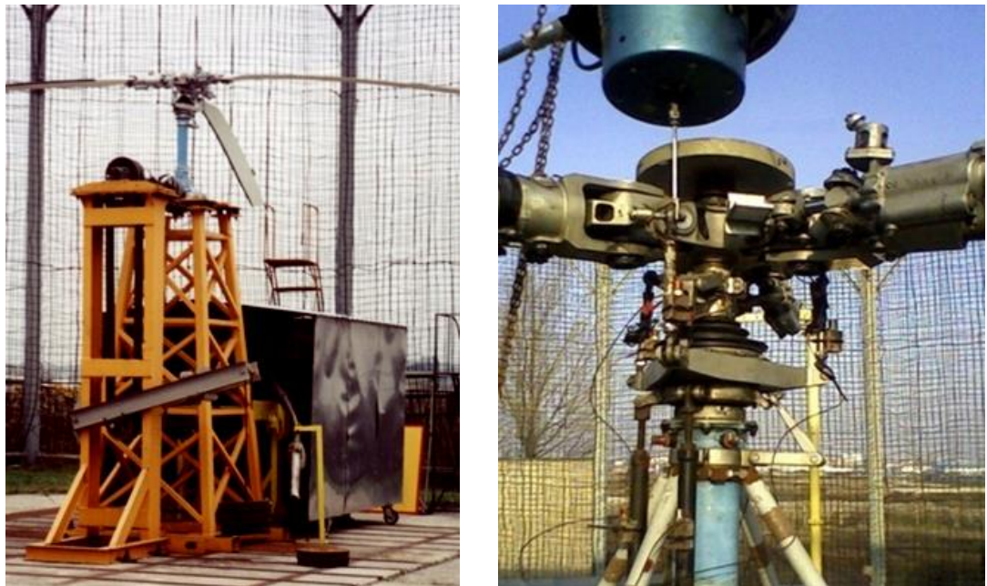
Fig. 4. The whirl tower system for helicopter three-blade main rotor [5]
