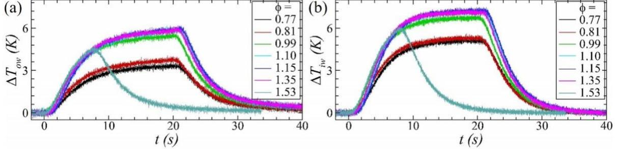
Fig 2. Cooling water temperature rises for 20-second tests with different equivalence ratios at (a) the combustor outer wall and (b) the inner wall. For all cases in this figure, both  $\dot{V}_{w,iw}$  and  $\dot{V}_{w,ow}$  are fixed at 45 l/min.
