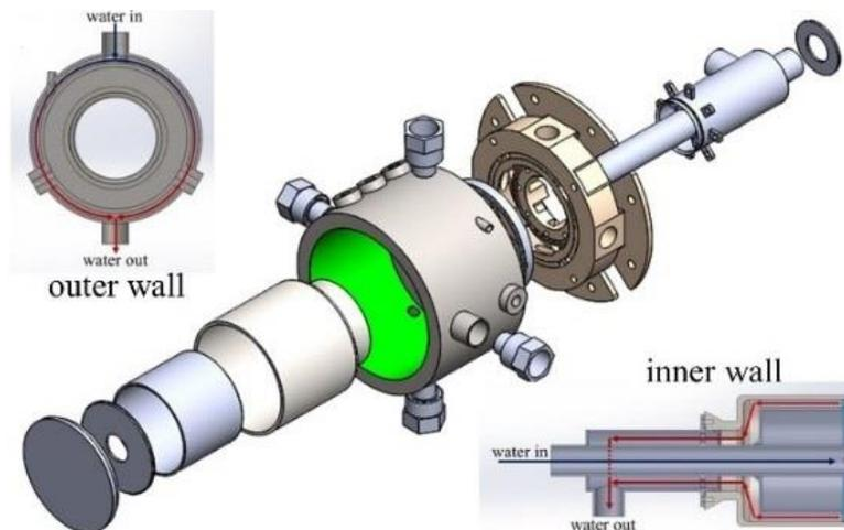
Fig 1. (a) A schematic drawing of the PGC with the water cooling jacket. (b) The experimental set-up of the water-cooled PGC.
