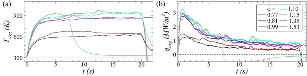
Fig 3. Moving averaged (a) temperature traces and (b) heat flux traces measure by the fast-response thermocouple for 20-second tests at different equivalence ratios. Both  $\dot{V}_{w,iw}$  and  $\dot{V}_{w,ow}$  are fixed at 45 l/min for all these cases.
