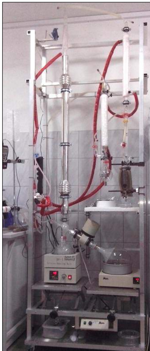
A system for concentration and purification of hydrogen peroxide
