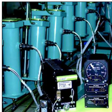
Stand for calibrating the PPM-1 fuelmeter system
