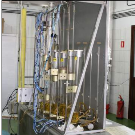
The test bed for calibrating the BPM-1 measuring and diagnostic system
