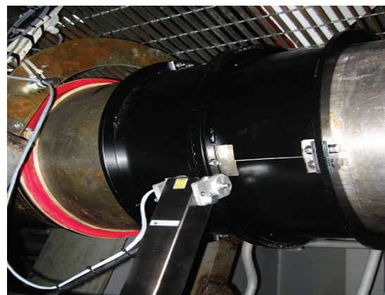
Fig. 2. Toothed rings and laser sensor mounted at intermediate shaft
