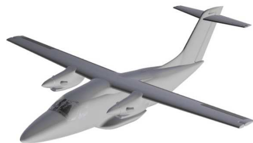
AC1 is a twin engine turboprop un-pressurized aircraft
